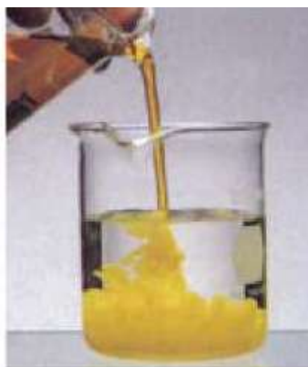
Figure 3.3 Lead (II) iodide precipitates when potassium iodide is mixed with lead (II) nitrate.
