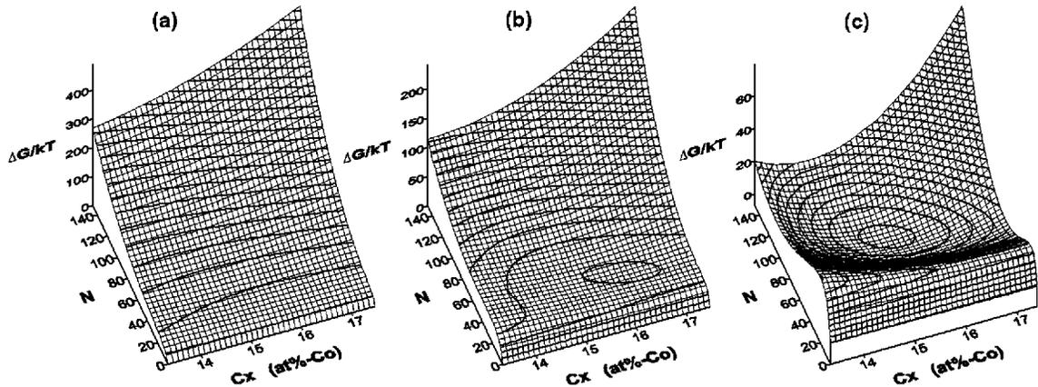
FIG. 5. Surface  $\Delta G(N, c_x)$  for the polymorphic mode without shape optimization ( $\varphi=1$ ) at  $\alpha=8 \times 10^{-18}$  J/atom for diffusion zone widths: (a)  $K=3.0$  nm; (b)  $K=3.5$  nm; (c)  $K=4.0$  nm. Here  $N$  is the number of atoms in the new phase nucleus ( $N=nv$ ) and  $c_x$  is the atomic fraction of species B at the center of the nucleus.
