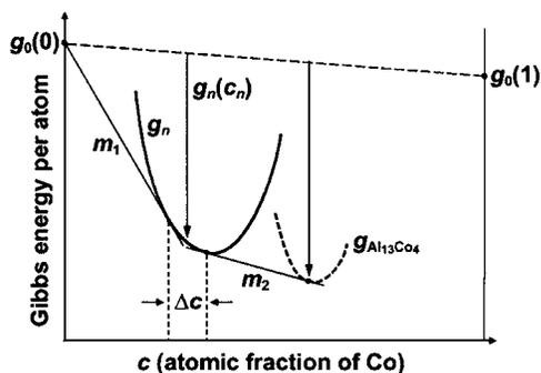
FIG. 8. Schematics of phase stabilities, Gibbs energies of phase formation, and equilibrium conditions of the terminating Al and the intermetallic phases  $\text{Al}_9\text{Co}_2$  and  $\text{Al}_{13}\text{Co}_4$ .
