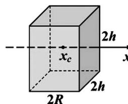
FIG. 2. New phase nucleus with the shape of a rectangular parallelepiped sized  $2R \times 2h \times 2h$  and its geometrical center at the point  $x_c$ . The concentration gradient in the parent phase is directed along the  $x$ -axis.
