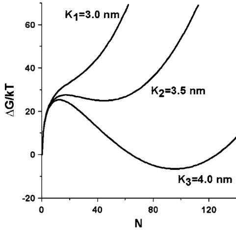
FIG. 6. Section through the  $\Delta G(N, c_x)$  surfaces for the polymorphic mode without shape optimization at a composition  $c_x = 15$  at %. ( $\alpha = 8 \times 10^{-18}$  J/atom, calculation for different diffusion zone widths:  $K_1 = 3.0$  nm;  $K_2 = 3.5$  nm;  $K_3 = 4.0$  nm.)
