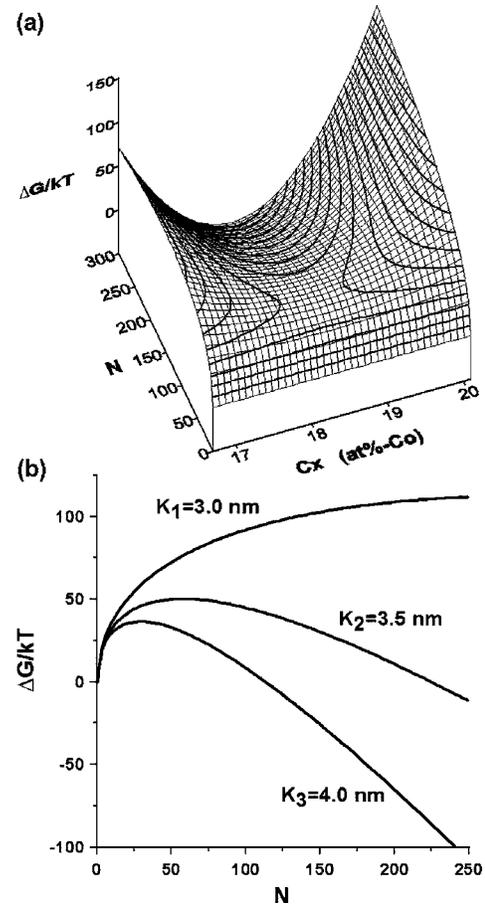
FIG. 7. Polymorphic mode with shape optimization at  $\alpha = 4 \times 10^{-17}$  J/atom: (a) surface  $\Delta G(N, c_x)$  for diffusion zone width 3.5 nm; (b) section  $\Delta G(N, c_x)$  at  $c_x = 18$  at % for diffusion zone widths  $K_1 = 3.0$  nm,  $K_2 = 3.5$  nm, and  $K_3 = 4.0$  nm. ( $N$  is the number of atoms in the new phase nucleus,  $c_x$  is the atomic fraction of species B at the center of the nucleus.)
