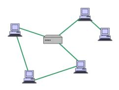
a ring, although two cable paths exist, messages can only travel in one direction.) Some WANs, most notably the Internet, employ mesh routing. A mesh network in which every device connects to every other is called a full mesh. As shown in the illustration below, partial mesh networks also exist in which some devices connect only indirectly to others.
