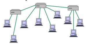
A tree topology integrates the star and bus topologies in a hybrid approach to improve network scalability.
