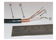
design in 1880. Coaxial cable differs from other shielded cable used for carrying lower-frequency signals, such as audio signals, in that the dimensions of the cable
