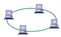
A ring topology such as FDDI or SONET sends messages clockwise or counterclockwise through the shared link. In a ring network, every device has exactly two neighbors for communication purposes. All messages travel through a ring in the same
